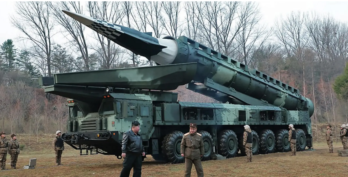
The Hwasongpho-16B on its TEL (with the clamshell at the front open)
